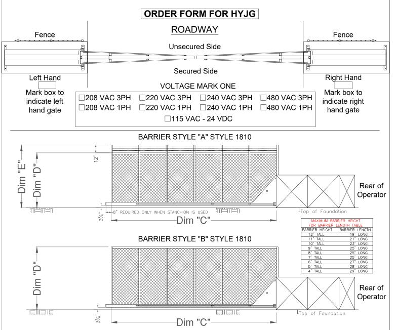
Note: Clearance between top of foundation and bottom of barrier is 3 3/4". If more or less is required, raise or lower foundation. Barriers 11 feet tall need 13 inches of clearance at rear of operator for barrier guard, and barriers 12 feet tall need 26 inches of clearance for barrier guard.
