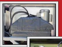
The TILT-A-WAY HYJG Series hydraulic gate operators have set the industry standard with their engineering, performance, and reliability. The 50" low profile pedestal houses a patented in-line balance system and a heavy-duty hydraulic operator. A 38" stroke hydraulic cylinder is assembled with a stout control rod alongside the cylinder rod. The cylinder is adjustable for optimal gate height at the far end of the barrier. When the gate is in the
